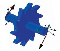
Detail Of The Total Constraint Forces On The Axle Of The Cogwheel
