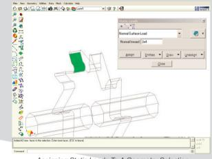
Assigning Static Loads To A Geometry Selection
